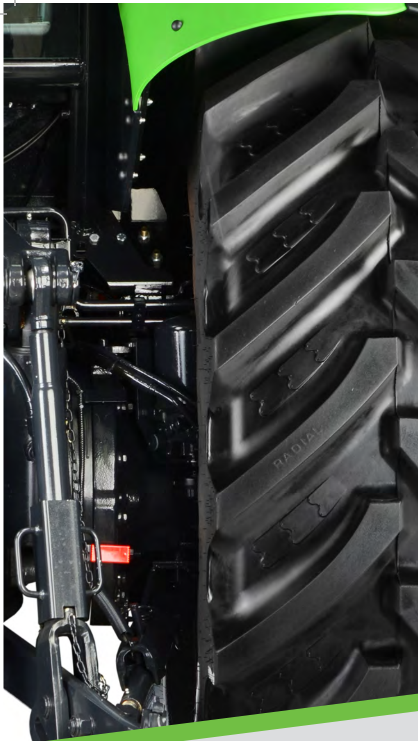
External rear lift and PTO remote controls from each side.
