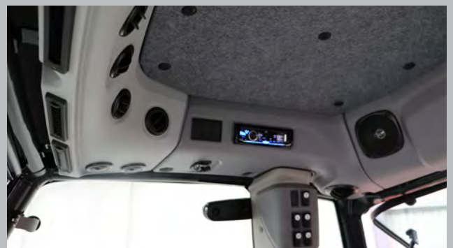
Air vents located throughout cabin.
